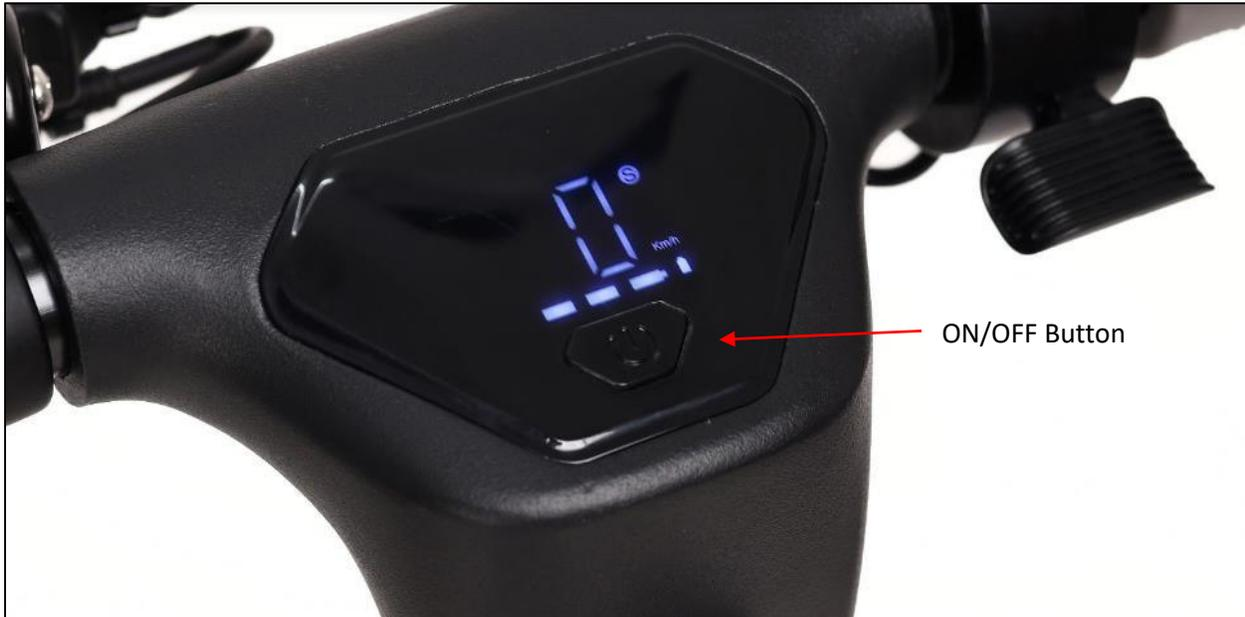
To turn your scooter on, long press the ON/OFF button until the display lights up and blink. Do not release the ON/OFF button until BLUE light stops blinking. Long pressing ON/OFF button again, will turn the electric scooter off.
